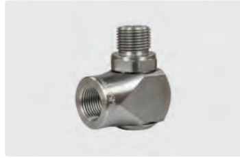
3/8" F : 3/8" M. Max. 400 bar / 30 tr/min / 90 °C
